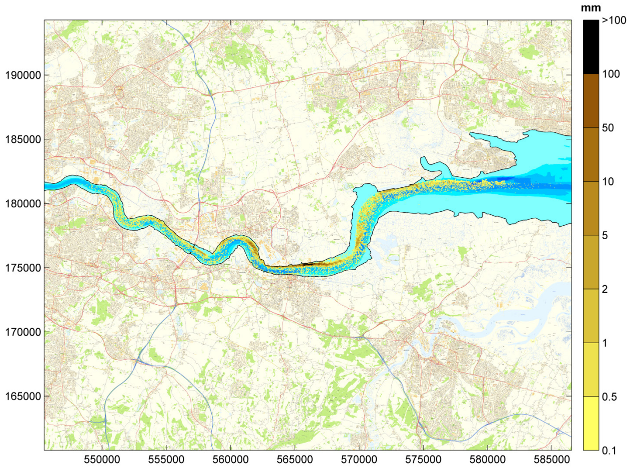
Figure 4.32: Maximum deposition depth of the released sediment during 5 days of dredging – Scenario 3
