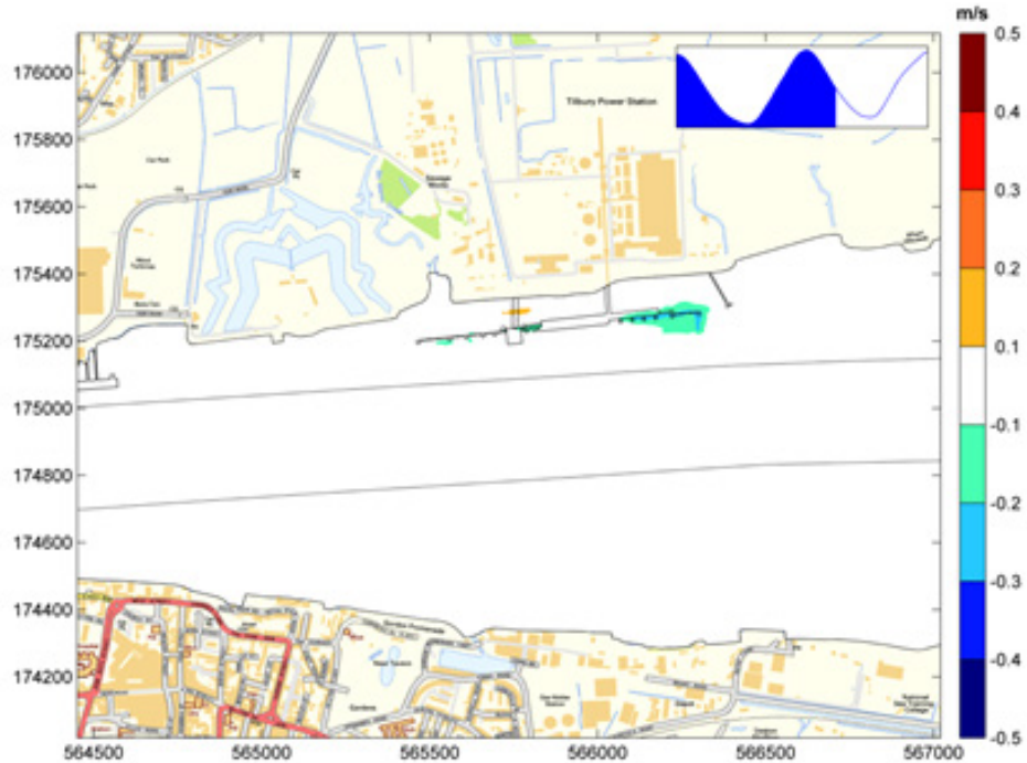
Figure 2.20: Difference in current speed magnitude - proposed works compared to baseline, near bed, peak ebb tide
